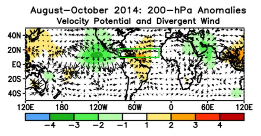
Figure 3: 200 mb anomalous velocity potential (10<sup>6</sup> m<sup>2</sup> s<sup>-1</sup>) and divergent wind for August through October of 2014. The green box indicates the Main Development Region. Anomalies are based on the 1981-2010 climatology. Figure courtesy of Gerry Bell (Climate Prediction Center).
