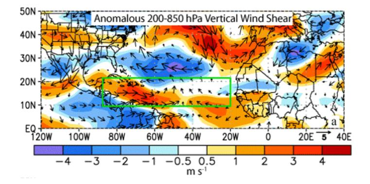
Figure 2: 200-850 mb anomalous magnitude of vertical wind shear and anomalous shear vector (m s<sup>-1</sup>) for August through October of 2014. The green box indicates the Main Development Region. Anomalies are based on the 1981-2010 climatology. Figure courtesy of Gerry Bell (Climate Prediction Center).
