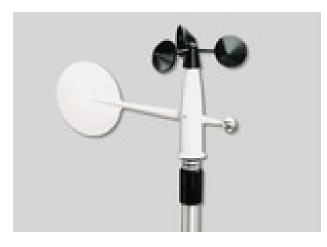
Obtaining accurate measurements of wind speed and direction requires considerable care. If your boat is pitching with the mast whipping through the air, the anemometer will reflect accelerations of the mast resulting in an erroneously high wind speed.
